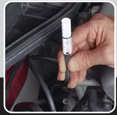
Flow meter quickly indicates presence of sealant
