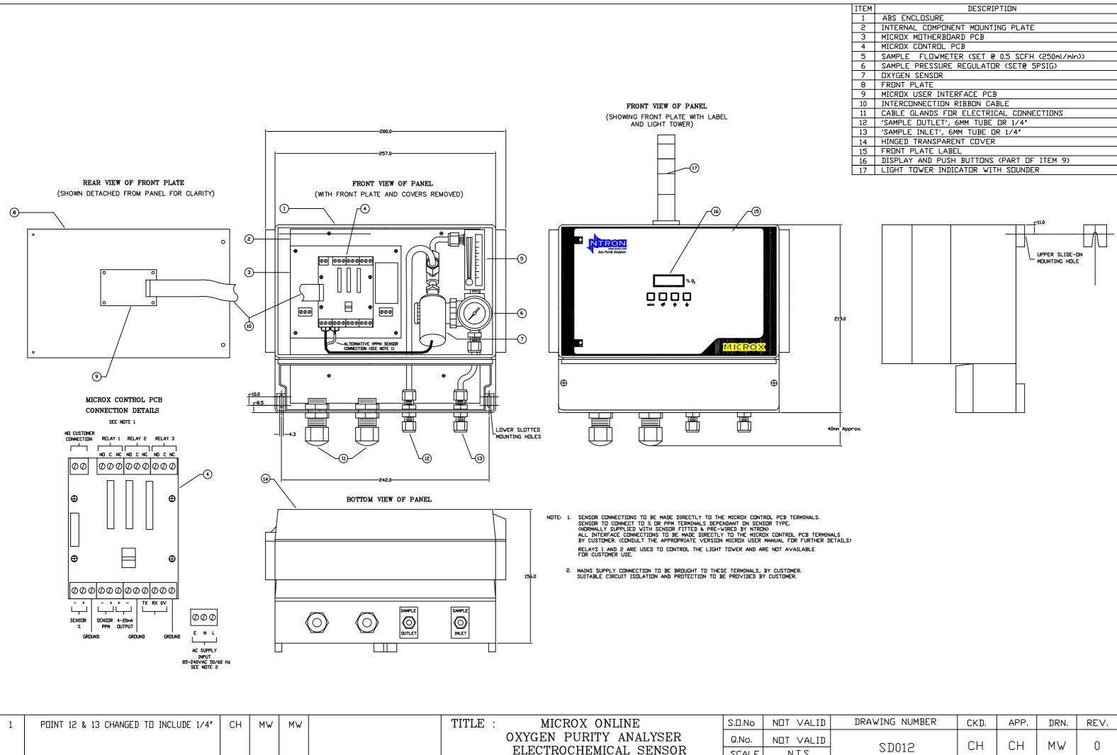
OXYGEN PURITY ANALYSER ELECTROCHEMICAL SENSOR DETAIL DRAWING
